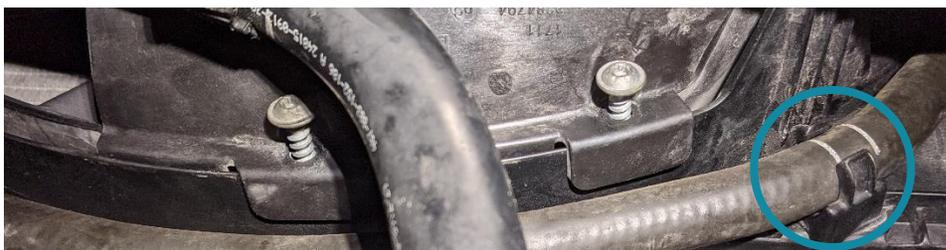
9. Next, drain the low temp (intercooler) water circuit, by disconnecting the lower hose from the intercooler pump:
