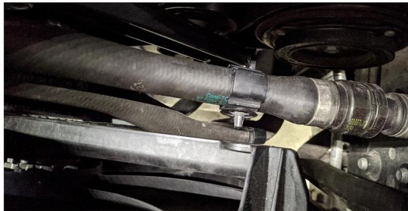
13. On the right side, remove the clip for the fan's electrical harness and then unplug the connector by squeezing the tabs on both sides:
