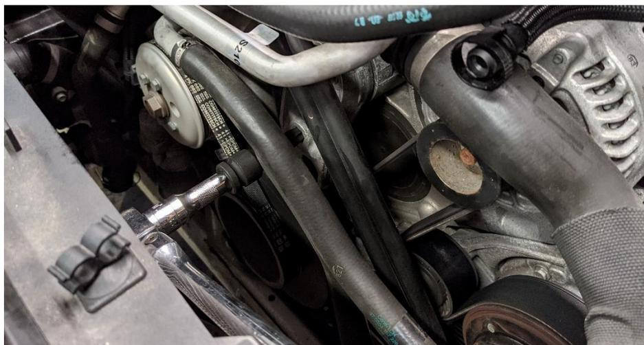
19. Remove the two lower idler pulleys to make room for the sealing cap removal tool:
