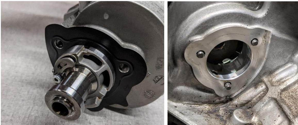
42. The Dorch Engineering vacuum pump assembly can now be installed in the block. Once it is seated in place, the timing gear needs to be placed back on the front of the shaft (reverse process of Step 37). This will require carefully using a screwdriver (again) to hold back the timing chain tensioner while the lining up the gear onto the front of the shaft.
