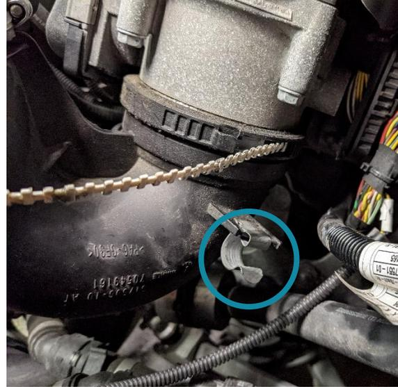
27. Prepare to remove the intake manifold by removing all electrical connections, clips, etc. that will be in the way. This includes the oil pressure sensor plug, rail pressure sensor plug, MAP sensor plug, and rear manifold bracket (2x T25 bolts pictured below, right).
