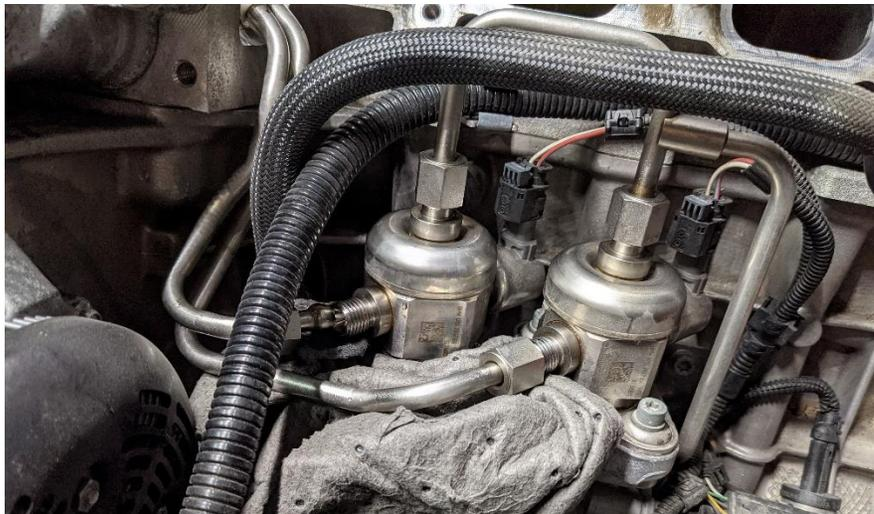
33. Now loosen the low pressure hardline hold-down clamps. Remove the two 13mm bolts below the cable junction assembly:
