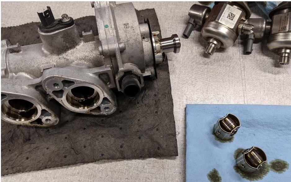
Once the pumps are removed, be sure to remove the cam followers (they just slide out vertically).
