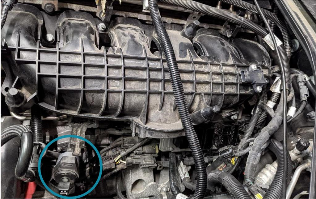
31. Now remove the intake manifold by loosening the 2x 11mm bolts and 5x 11mm nuts. It requires some maneuvering, but it will come right out.
