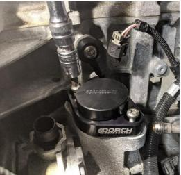
19. **BEFORE** inserting the HPFP into the flange, push the low pressure hose on to the Dorch HPFP inlet. You will need to unthread and remove the locking collar, slide the hose onto the pump, and then re-install the locking collar. The HPFP can then be dropped into place in the flange.
