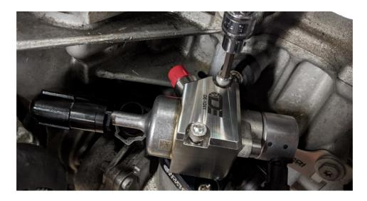
21. The low pressure hose can now be routed into it's final position and clipped into the OEM hose. The Dorch low pressure hose simply slides right into the OEM BMW hose. It may take some effort, but it will click in. Once it clicks in, it will not pull out. The gray clip can then be re-installed on the OEM BMW hose (Ref. Step 15).
