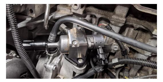
25. At this point double check all of your fuel connections, fastener torques, etc. and then the reassembly process can begin. Re-install everything just as it came off. We recommend new throttle body and intake manifold gaskets upon reassembly.
