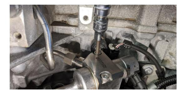
Lightly apply oil to the threads of the HPFP to prevent galling. If the nuts thread on effortlessly and bottom out with all the fittings well aligned, the nuts can now be torqued (a 17mm wrench can be used for this if need be, since special sockets are required for proper torque). Be sure not to over tighten the nuts.
